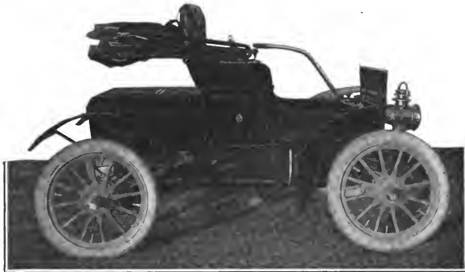
OLDSMOBILE 7-HORSEPOWER RUNABOUT WITH PIANO BOX BODY AND STRAIGHT DASH.
